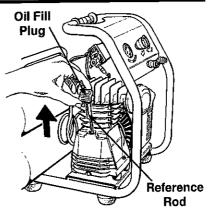
necessary add oil (See "Assembly/ Fill Pump with Oil" section of this manual)
